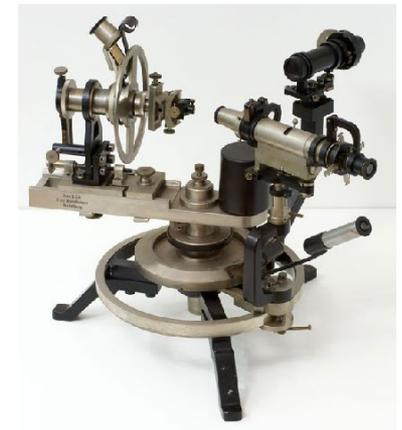
Apparatuses to measure an angle which two faces form
