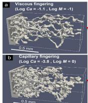
CO<sub>2</sub> behavior within the rock pore at different conditions via fluid flow simulation
