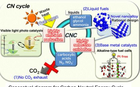
Conceptual diagram for Carbon-Neutral Energy Cycle
